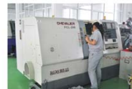
进口高精度斜导轨数控机床 Imported high-precision slanted guide rail numerical control machine
